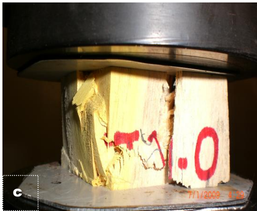
Fig a-d: Photographic views of Progressive stages of plastic deformation of wood specimen along the grains
